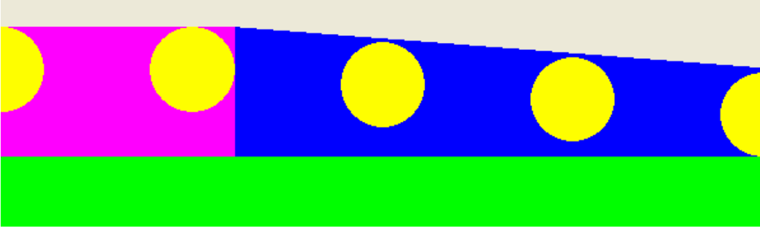
Figure 3 Printing with a high EOM stencil. Note that mesh threads are not in contact with the substrate towards the image edge.
