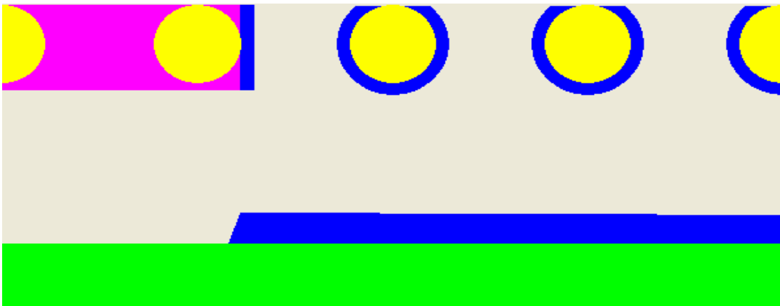
Figure 2 The same system after the mesh has lifted off the substrate
