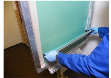
There are obviously many variations to the coating regime depending on frame size, mesh count, image requirements etc. but the principle requirement is always to start the base coats from the print side and finish on the squeegee side.
